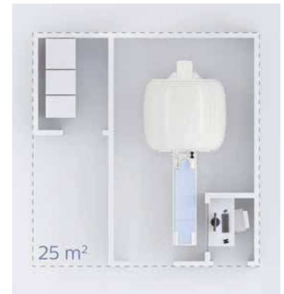
Console room in this illustration is outside of the 5 Gauss line. Minimum site layout is for illustration purposes only. For detailed site planning please contact your Philips representative.
